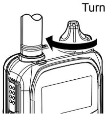
① The dial is made tight for the dust and water resistance.
