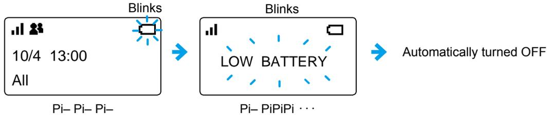
①When “LOW BATTERY” is displayed and beeps sound, the transceiver power will be automatically turned OFF soon.
