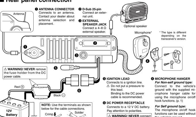
ground with the supplied microphone hanger cable for using the microphone on/off hook functions. (p. 1)
