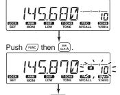
Rotate  $\frown / \bigcirc$  to select the memory channel.
