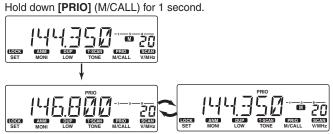
The watch checks for a signal on memory channel 20, every 5 seconds.
