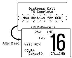
② After receiving the acknowledgment, reply using the microphone.
