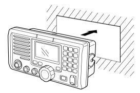
$\ \, \ \,$  Attach the 2 supplied bolts (M5  $\times$  8 mm) on either side of the IC-M603.
