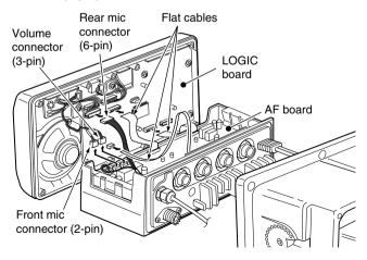
③ Install an optional unit to J3 on the AF board as shown below.
