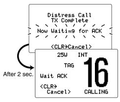
4 After receiving the acknowledgment, reply using the microphone.
