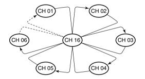
Priority scan searches through all TAG channels in sequence while monitoring Channel 16. When a signal is detected on Channel 16, scan pauses until the signal disappears; when a signal is detected on a channel other than Channel 16, scan becomes Dualwatch until the signal disappears.
